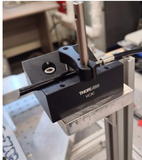
Fig. 6 Optical sensor mounted to thrust stand assembly
